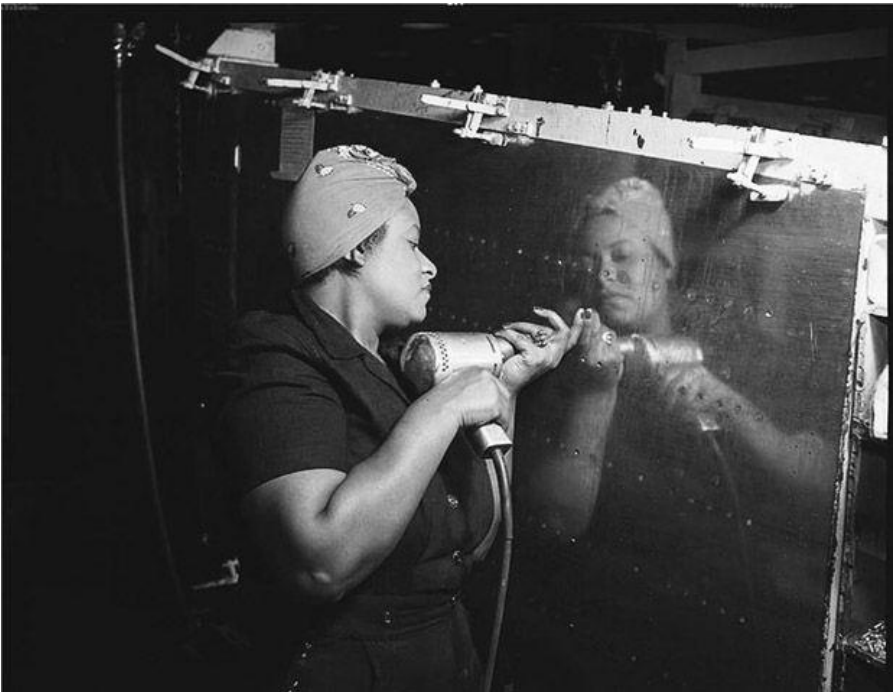
Working a hand drill at Vultee-Nashville, Tennessee, on an A-31 Vengeance dive
